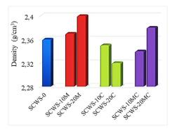
Fig. 6. Variation of density versus substitution rate
