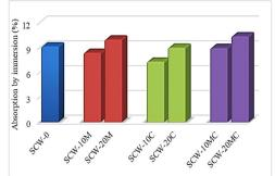
Fig. 13. Change in the immersion absorption coefficient as a function of the substitution rate
