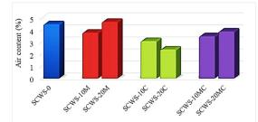
Fig. 7. Change in air content as a function of the substitution rate
