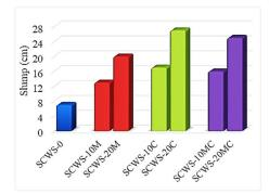
Fig. 5. Variation of workability as a function of the substitution rate
