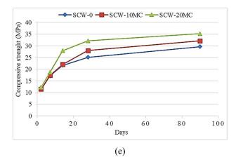
Fig. 9. Compressive strength of concretes studied as a function of time
